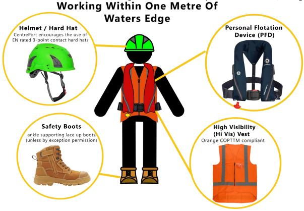
Anyone working within 1 metre of the edge of a wharf or water's edge is required to wear a Personal Flotation Device (auto-manual self-inflating).
